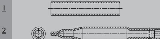
Tube produced by infeed and plunge swaging, right end formed over a mandrel.
