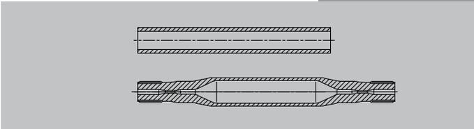
Example of a part produced by the HMP upset swaging method.
