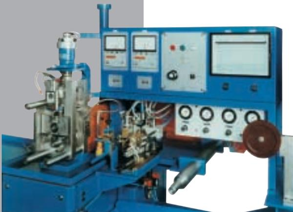
HMP manufactures precision rolling machines for flat rolling and profile rolling. The machines may be equipped with one, two, or more stands.
